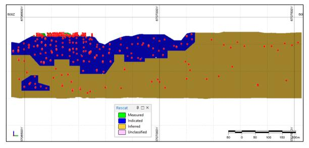
Figure 5 Isometric View (looking down towards the NE) showing classification of mineralised lodes
